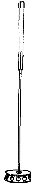
Nelson stirring-rod and cream sampler. (Invented by N. C. Nelson, station operator, Eskridge, Kan.)
