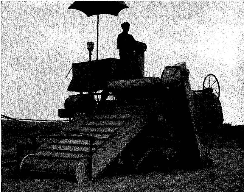
FIG. 17.—The Fort Hays experiment station grass combine with low-cutting attachment for harvesting buffalo grass seed.
